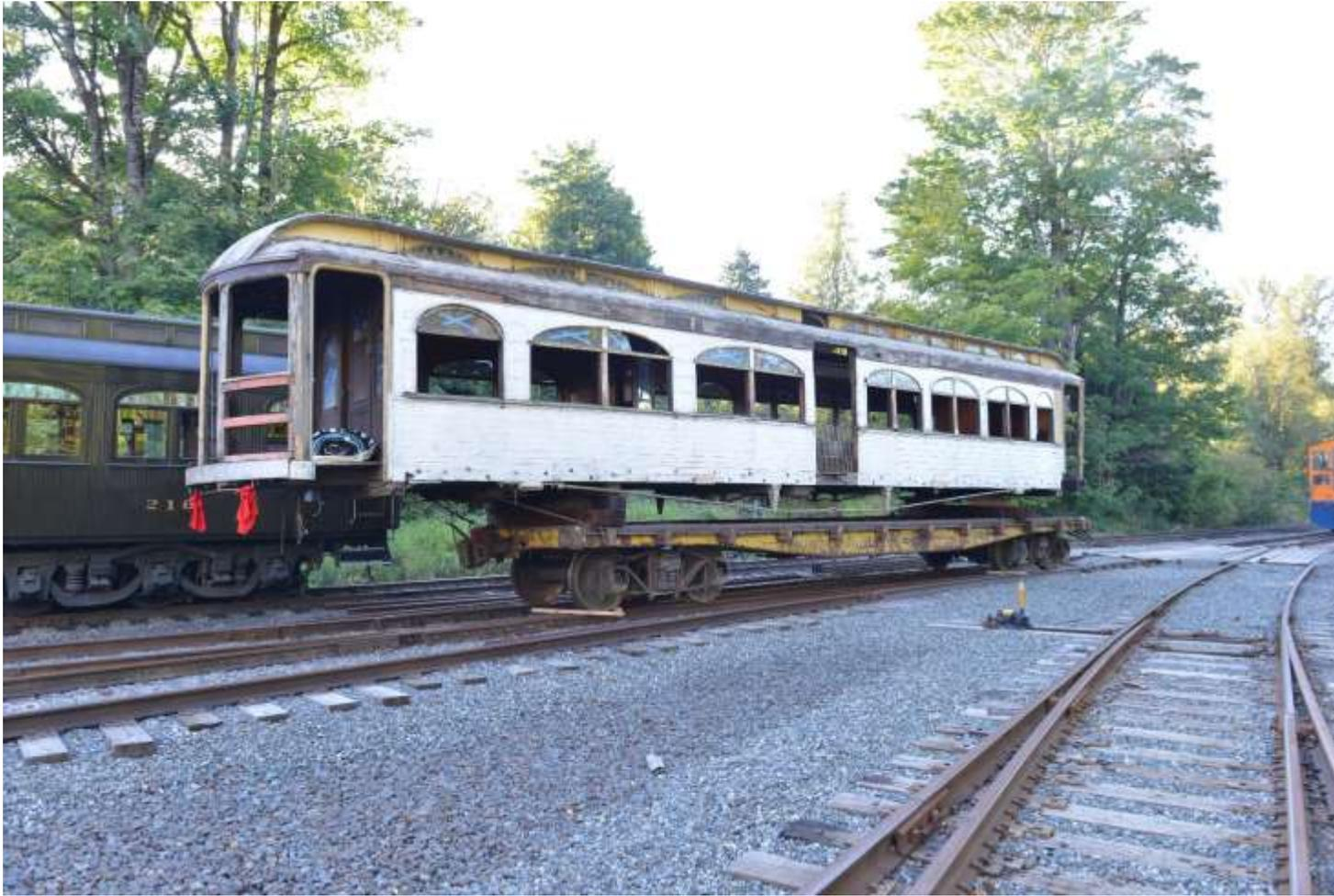
This is the right side of the car. The end closest to the camera is the rear of the car. The opening in the center is where the residential doorway was cut into the car side. Post 1910 there was no restroom on this side of the car. (In this view, 523 is sitting on a railway flatcar to facilitate its movement around the museum.)
