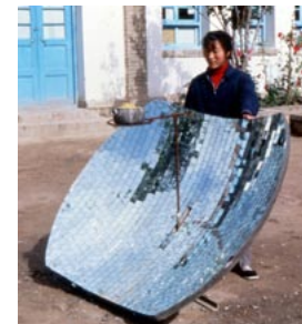
"Green Tea" - Solar boiler manufactured at collectives in China and made available to field laborers to cook and boil water in the 1980's.
